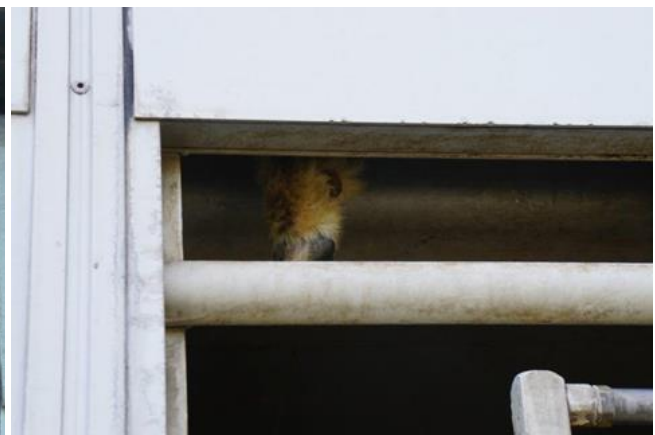
Trapped leg – vehicle with high risk for injuries
