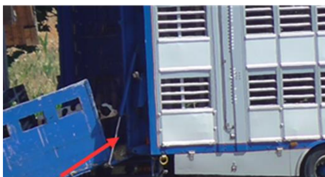
Loading: Gap between the ramp and the door
